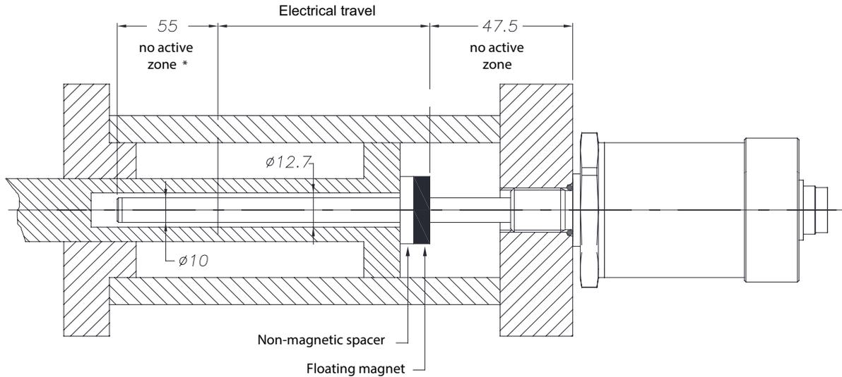
\* for stroke up to 1000 mm (included) – over 1000 mm, the non-active zone becomes 60 mm because the tip includes a M4 threaded hole
