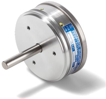
The RPS50 potentiometers with servo flange housings are for applications where a very precise wirewound potentiometer with high electrically effective rotation angle is required.
