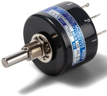
The potentiometers OMCP are filled with oil. The oil has a heat-dissipating function, cleans the resistance element of abrasion and protects it from moisture and aggressive substances.
