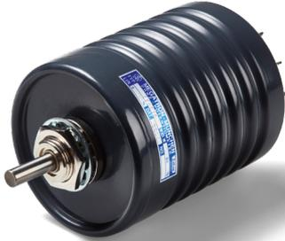
The potentiometers OF50 are filled with oil. The oil has a heat-dissipating function, cleans the resistance element of abrasion and protects it from moisture and aggressive substances.
