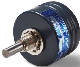
The potentiometers OF5001 are filled with oil. The oil has a heat-dissipating function, cleans the resistance element of abrasion and protects it from moisture and aggressive substances.
