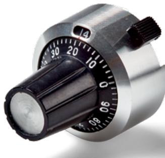
The knob SKK with 50 dashes and revolution counter (20 rev.) in Ø22 mm housing has a locking mechanism and a cardan coupling.
