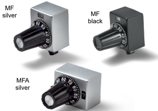
**Miniature adjustment knob MF in 18.5 x 15 mm housing with 50 dashes, revolution counter (10 rev.), locking mechanism and cardan coupling.**
