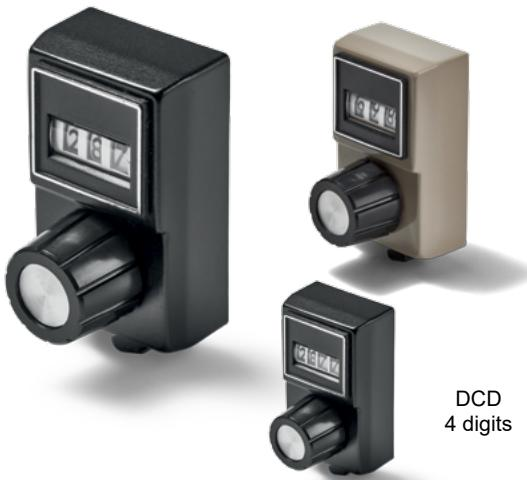
**Adjustment knob DCD in 26 x 44 mm housing with 3 or 4 digit display for 10 or 100 revolutions and locking mechanism.**
