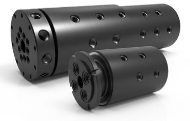
GP models with 2, 3, 4, 6 or 8 flow passages come standard with NPT thread shaft connections and O-ring face seal glands for flush mounting the union to an interface. GPM (metric) models with BSPP connections are not available with O-ring face seal glands.
